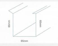
CARBOLITE bullnose gutter attachment
