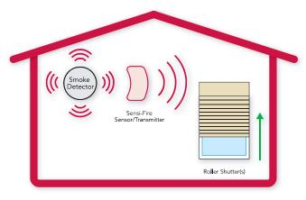
Installation Requirements: The Sensi-Fire Wireless receiver/ transmitter must be positioned within 500mm of a working smoke detector that meets Australian Standards.
